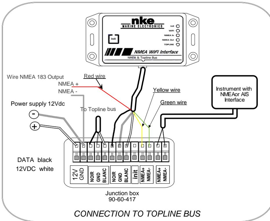
Should you need to shorten the bus cable, uncover and tin the wires before connecting in the junction box.
